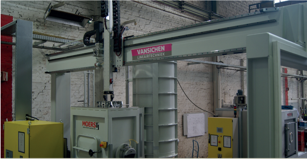
AT35-XZ system with Z-axis from aluminum AT35-XZ System mit Z-Achse aus Aluminium
