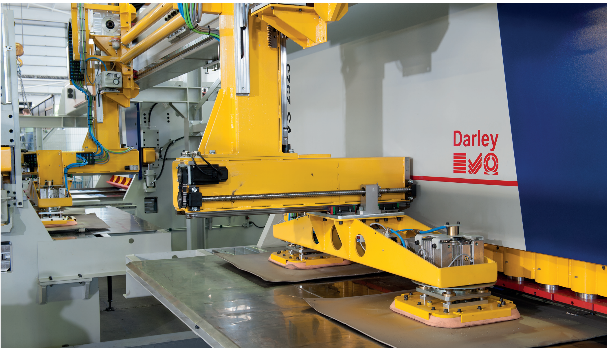
Handling system to manipulate nickel plates Handling Systeme um Nickel Platten zu manipulieren
