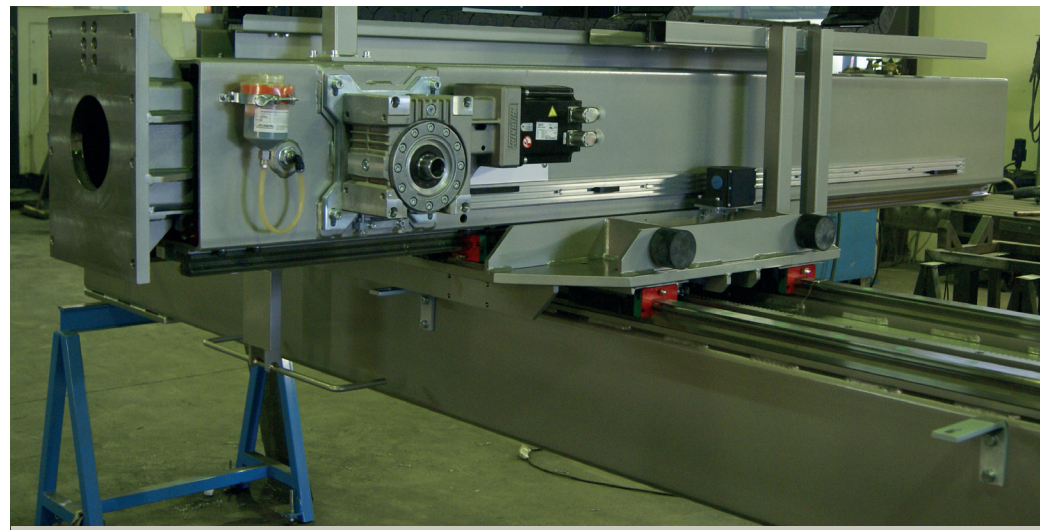
Telescopic Y-axis. Hub 2500 mm, stroke 68000 mm Teleskop Y-Achse. Hub 2500 mm, Schlag 68000mm
