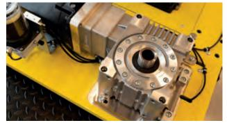
**1. LOW BACKLASH GEARBOX**Planetary gearbox as an option // Motor sizing assistance
